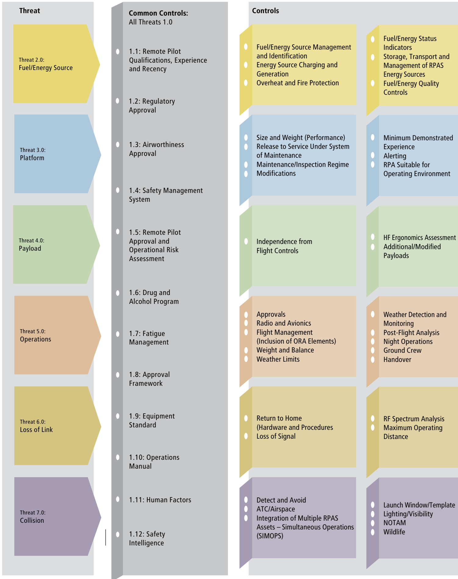
Figure 1: BARS Bow Tie Risk Model – Schematic of Remotely Piloted Aircraft Systems Management
