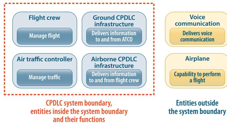
**Figure 3: Controller-Pilot Data Link Communication (CPDLC) system**
